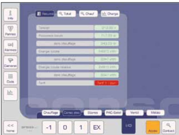
On the display, the users can view details of energy consumption (shown), heating parameters, and air quality data.
