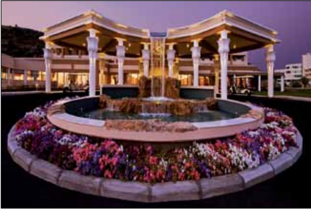
Stylish waterfall: To prevent a gust of wind from blowing the water in the wrong direction, a KNX weather station switches off the pump when the wind is too strong.
