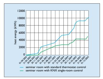
**Figure 2.** The logged data of the comparison test covered the periods from the beginning of 2002 until the end of 2005. However, the rooms weren't fully used until the middle of 2004. The "KNX controlled" room could save up to 50 % of the energy as compared to the "normal" room.
