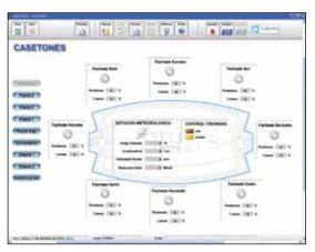
Visualisation example: The menu page of the weather station provides information about the external temperature, brightness, wind speed and solar radiation as well as the status of the eight façade sections.
